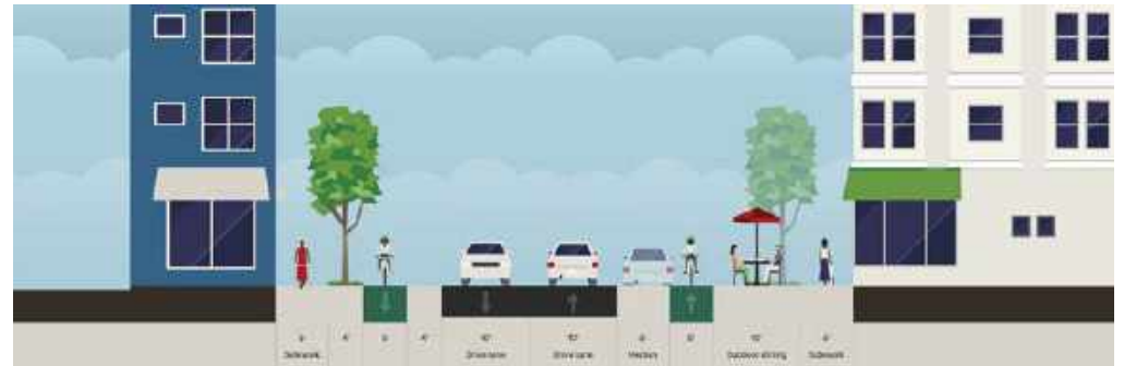
Proposed Street Section Villard Corner
