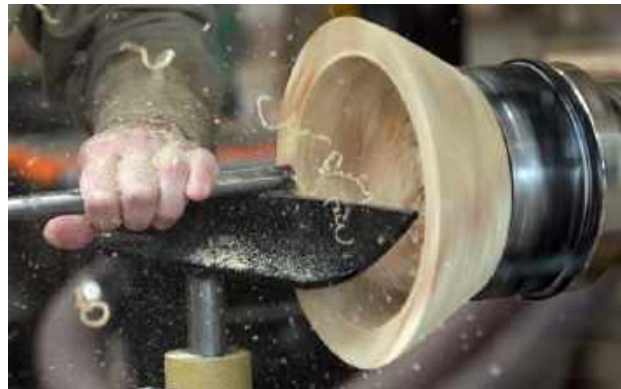
Turning a bowl on the lathe
